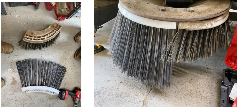
WO062823006 Street Sweeper replacement of the brush heads.
