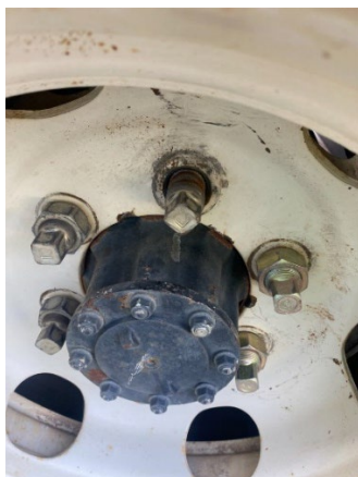
WO061923004 Emergency repair on the Street Sweeper lug nuts.
