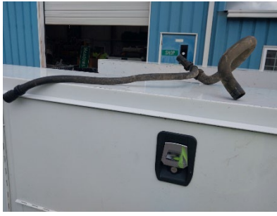
WO062023001 Replaced coolant hose on truck 1333
